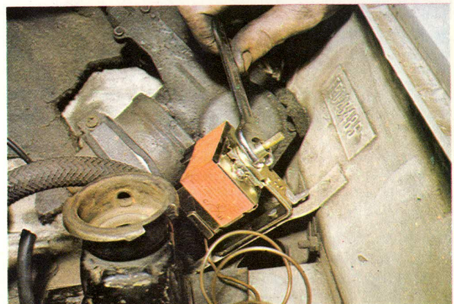
28 Fix the control unit on to the bracket, screwing the half-nut on to the spindle. The copper capillary must run down behind
