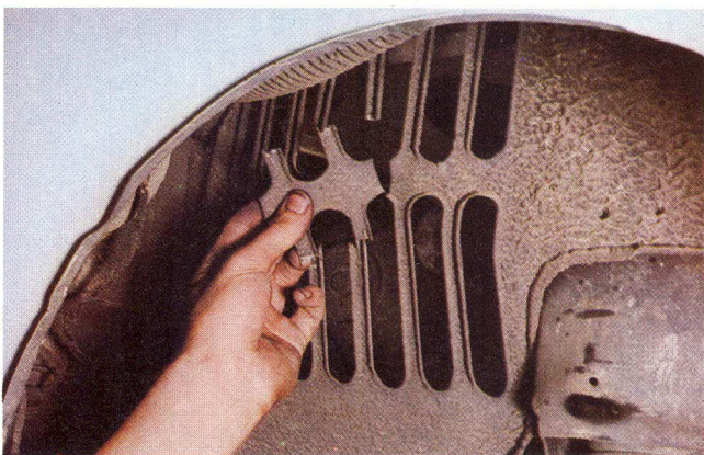
4 Carefully remove the sawn-out section and discard it. It is a good idea to file down any jagged edges left around the hole
