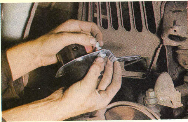
6 On this Mini 1275GT, there is only one mounting bracket. This is bolted to the motor loosely, leaving some room for adjustment
