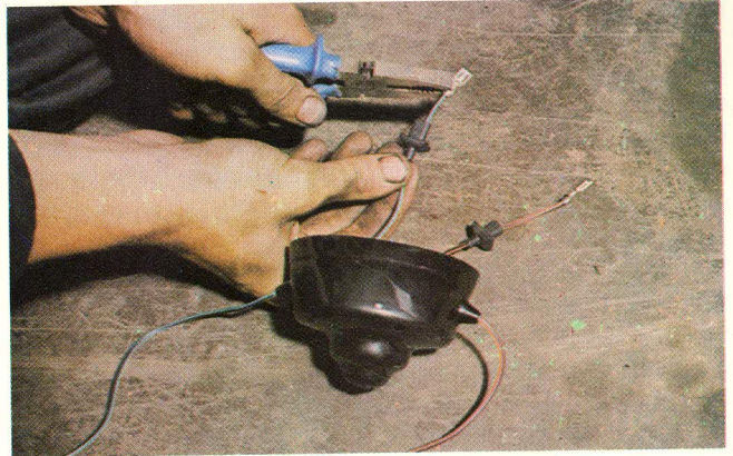
9 When connecting the motor wires, feed them through the plastic cover and the shrouds before crimping on the spade connectors
