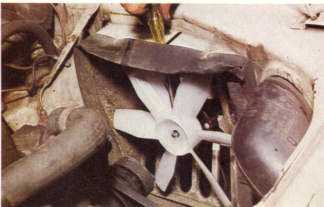
16 Fix on the fan blade from inside the engine compartment. Screw down the fixing screw tightly and then check for fouling
