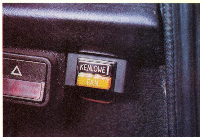
34 The switch in place on the fascia. Whenever the fan starts up the warning light comes on, whether the switch is on or off
