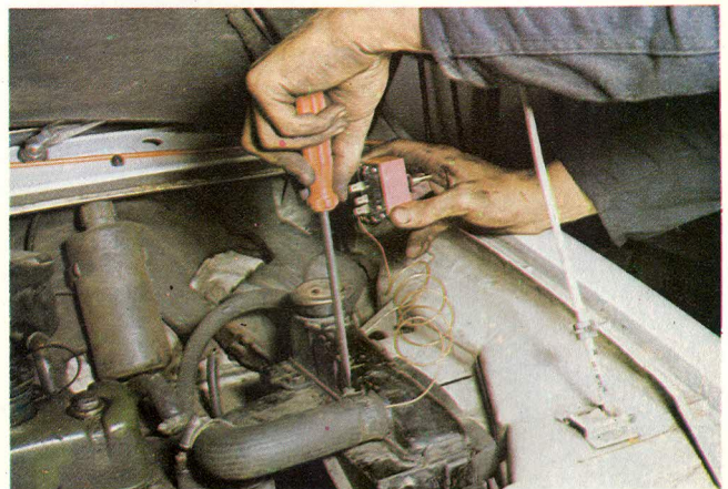
26 With the thermal control sensor inserted into the radiator and the rubber seal in position, tighten the clip on the top hose
