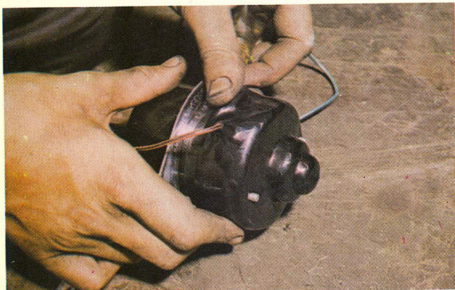
12 Having completed the test and changed the wires if necessary slide the plastic waterproof cover right over the motor body
