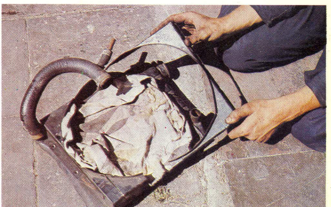
17 To cut down the radiator cowling, start by removing the upper part, held by four bolts. It can then be worked on on the bench
